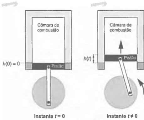
A função  $h(t) = 4 + 4\text{sen}\left(\frac{\beta t}{2} - \frac{\pi}{2}\right)$  definida para  $t \geq 0$
