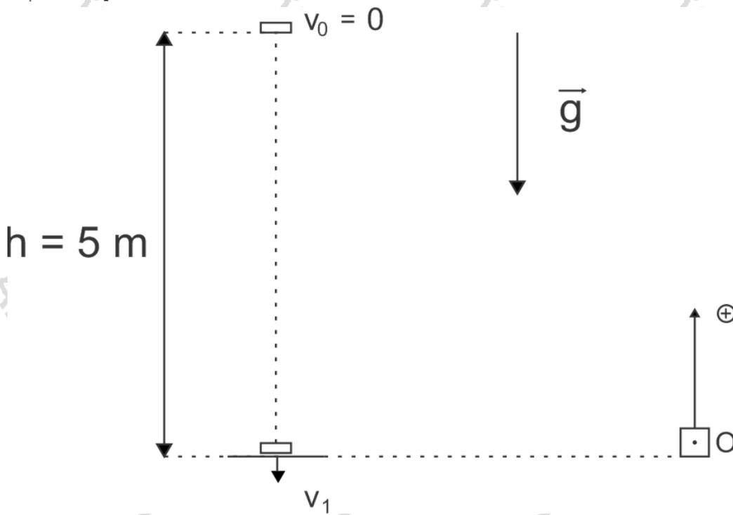
$$\begin{aligned}v_1^2 &= v_0^2 + 2 \cdot a \cdot \Delta s \\v_1^2 &= 2 \cdot (-10) \cdot (-5) \\v_1^2 &= 100 \Rightarrow |v_1| = 10 \text{ m/s}\end{aligned}$$
